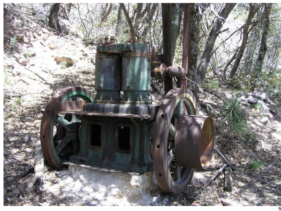
75HP Engine to Drive Compressor
